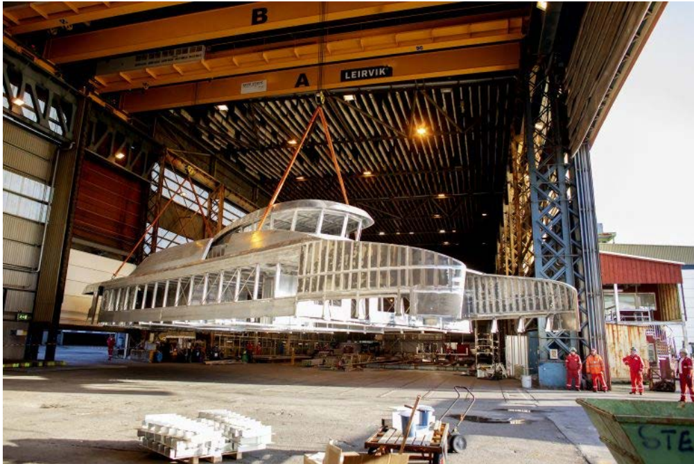
Figure 1. Medstraum's main structure (Fjellstrand shipyard) (source: https://www.fjellstrand.no/ )
