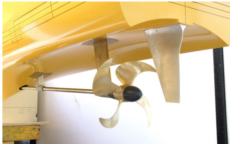
Figure 14. View of the stern area of the tested Stavanger model, with fitted propellers, shafts, brackets and rudders
