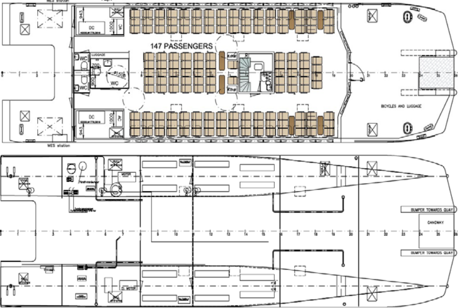
Figure 7. Initial general arrangement of the Stavanger Demonstrator
