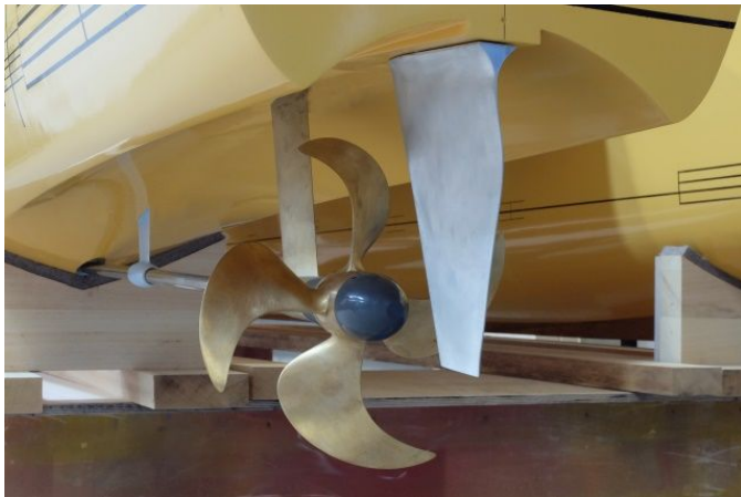
Figure 21. View of the tested Stavanger model
