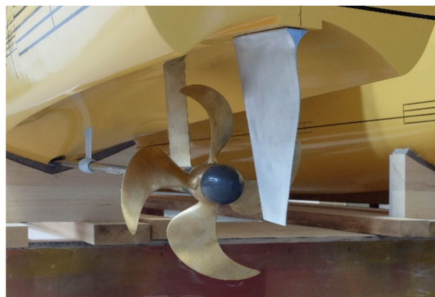
Figure 6. Close-up of the transom stern area of the tested Stavanger model, with fitted propellers, shafts, brackets and rudders [34].
