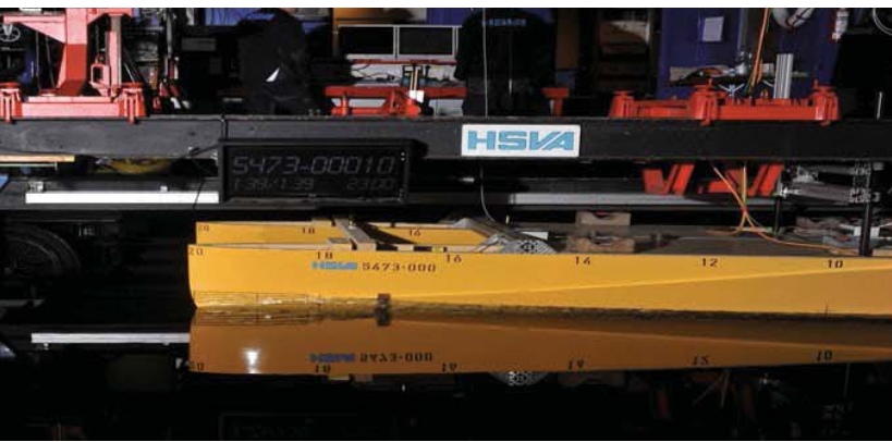
Figure 8: Self-propulsion model of the Stavanger demonstrator at 23 knots full scale speed
